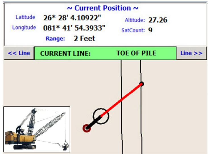
During setup the user will enter the distance from the tip of the boom to the location of the GPS antenna array. The software then generates a real-time representation of the vehicle's boom. If production lines - such as the "toe of pile" line pictured above - are entered into the system, the distance from the tip of the boom to the currently selected line is automatically calculated and displayed on the screen.
