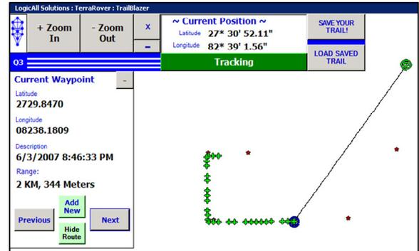
The operator interface displays the current location, the destination, and the distance between the points. A routing line indicates direction to travel to reach the selected waypoint. Ideal for any situation where you need your resources moved to specific locations. Waypoints may be assigned remotely and loaded or the user may record their current position as a waypoint.
